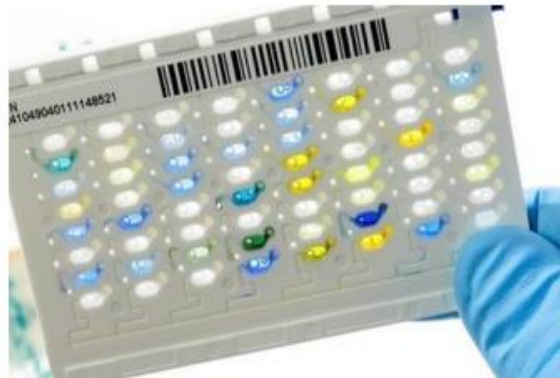
Fig 3: identification cards are used for isolation and identification of bacteria in vitek 2 machine
