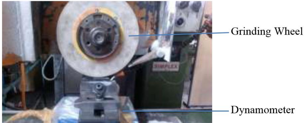
Fig 1: Grinding machine experimental setup
