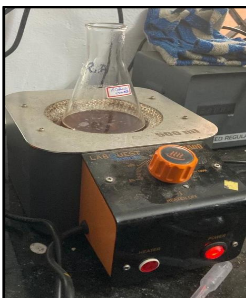
Figure 4: The Extract Solution which was Kept in a Conical Flask was now Heated with the Help of Heating Mantle for 5 minutes at 70 Degree Celsius
