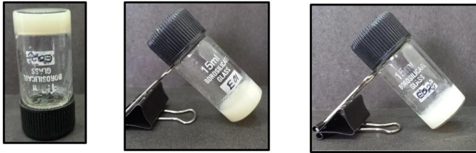
Figure 2: Optimization of Gelation with Different % Clove Oil Loading with 2 % of Cross Linker A) 0.5 % Oil Loading; B) 10% Oil Loading: C) 2% Gel Loaded with 10 % w/v of Nano HAP Particles and Clove Oil
