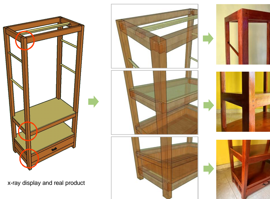
Figure 5: Three main wood joints
