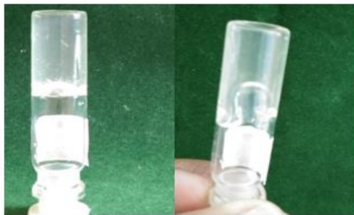
Figure 3: Hydrogel on day 3 followed by day 5(3% chitosan with 0.125%gluteraldehyde)
