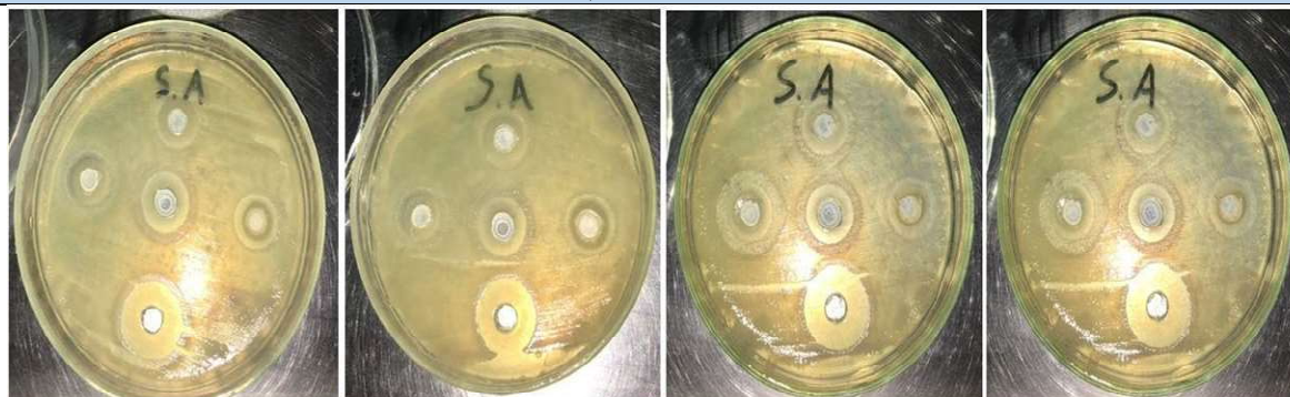
Figure 3. Inhibition halos (in mm) placed by the tested materials in function of the Staphylococcus aureus in aerobic condition measured in 24, 48 hours, 1 week and 2 weeks.
