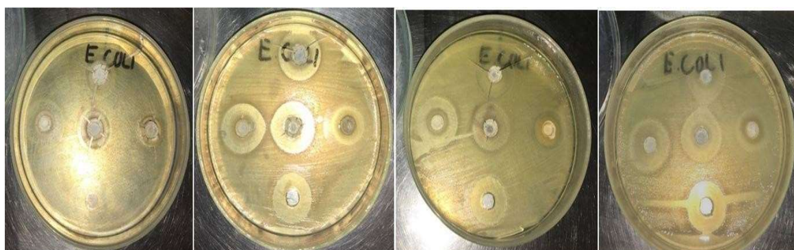
Figure 1. Inhibition halos (in mm) placed by the tested materials in function of the Escherichia coli in aerobic condition measured in 24, 48 hours, 1 week and 2 weeks.
