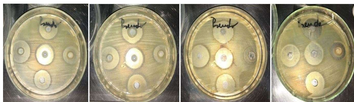
Figure 2. Inhibition halos (in mm) placed by the tested materials in function of the Pseudomonas aeruginosa in aerobic condition measured in 24, 48 hours, 1 week and 2 weeks.
